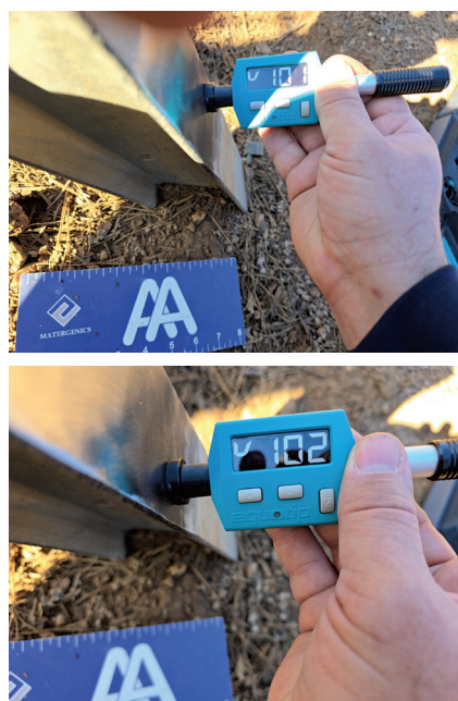
Fig. 10 — Photographs showing Vickers hardness values of anchor AA (flange).
