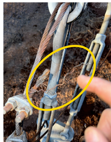
Fig. 11 — Small strand sample from wire rope at anchor BB removed for examination.
