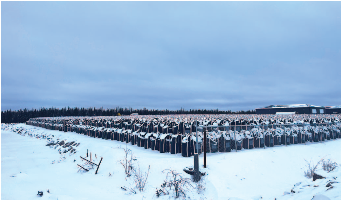
Large quantities of cement have to be stockpiled in Yellowknife, as the material can be transported to mine sites only when the ice roads are available for a couple of months each year.
