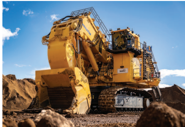
The PC9000 shovel during assembly and testing at Suncor’s Fort Hills mine.
