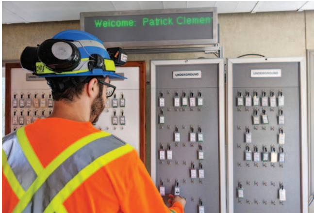
TopVu's eTag Board sends worker information to TopVu's web-enabled Q7 software.
