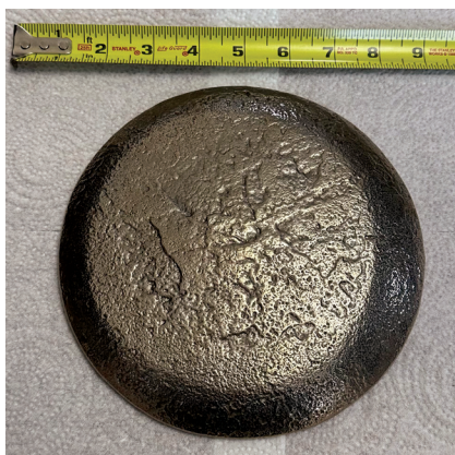
Fig. 6 — As-cast bun, bottom surface.
