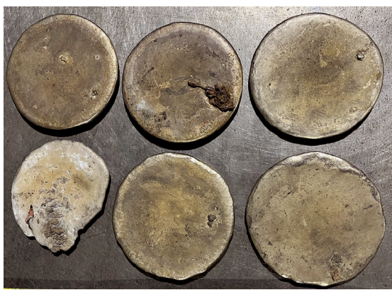
Fig. 8 — Casting defects observed on buns.
