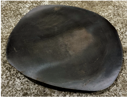
Fig. 12 — Cymbal blank, finished size, as-rolled. (15-in. diameter, 0.050 – 0.053-in. thickness)
