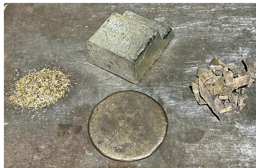
Fig. 4 — Copper scrap (left and right) and tin ingot (top) for producing a high-tin bronze bun (bottom).
