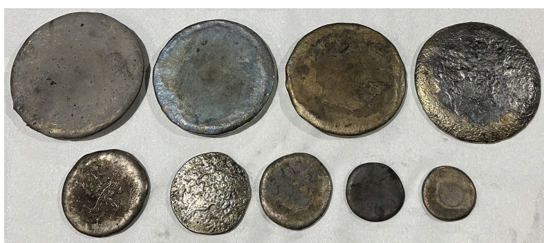
Fig. 9 — Bronze buns exhibiting surface conditions relating to pour temperature and cooling rate. Top row from left: Bun 1 temperature too low at pour; bun 2 and bun 4 exhibit tin-rich phase at surface (inverse segregation); bun 3 color suggests low Sn content. Bottom row: Various smaller cast buns for finger cymbals or medallions.
