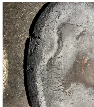
Fig. 7 — Hot-worked blank exhibiting edge cracks; as-rolled, first pass.
