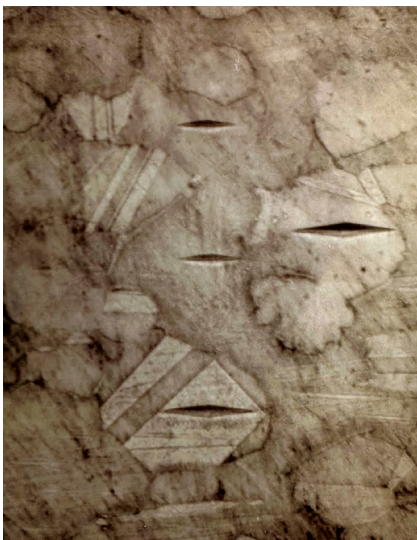
Fig. 13 — Cymbal blank microstructure; finished blank, as-rolled and quenched, 75x. Twinning, 77 HRB, matrix, 39 HRC (converted: HK 25-gram load). Courtesy of Fredrick A. Skinner, metallurgical consultant.
