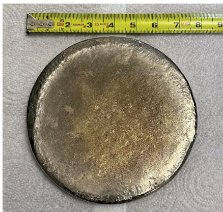
Fig. 5 — As-cast bun, top surface.
