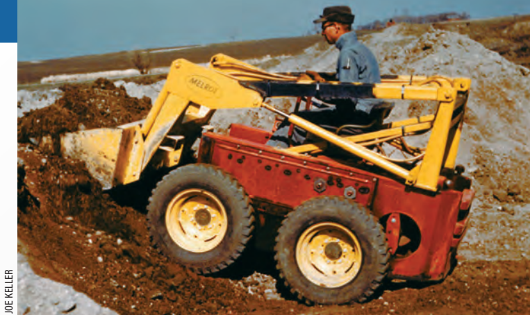
Louis Keller operates the first M440 prototype, which featured a more robust design and was the first to have closed drive compartments and double-acting hydraulic lift cylinders.
