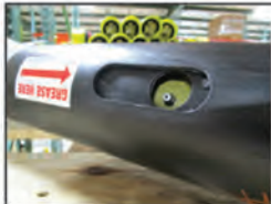
Patent Lever Release Safety Guard with quick release clamshell guard on all CV shafts
