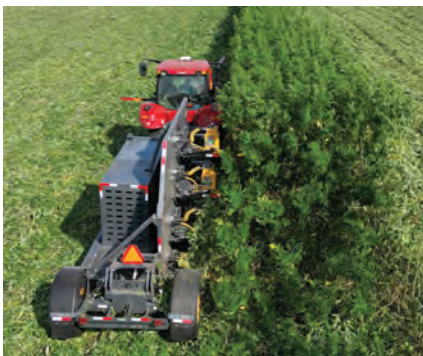
John Peterson uses a Bish FiberCut to cut tall industrial hemp stalks into several more manageable pieces.
