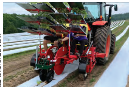
Mechanical Transplanter Co. offers carousel- and finger-style transplanters for planting CBD hemp in bare ground or plastic mulch/film. Pictured here is the Model 948 Mulch Transplanter.
