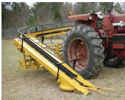
The Powell 6031 Hemp Harvester cuts CBD hemp plants at near ground level, and then properly orients them and sends them up a conveyor to a wagon or trailer pulled alongside the tractor-drawn harvester.
