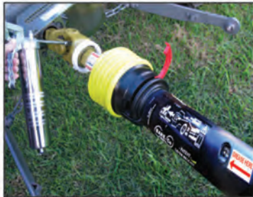
Patent Lever Release Safety Guard with quick release clamshell guard on all CV shafts
