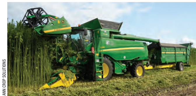
CANN Crop Solutions provides equipment that can harvest every part of an industrial hemp plant. Its DoubleCut Combine (pictured) can harvest and separate a complete plant. “That gives the cleanest product streams possible, leading to higher-quality fiber, seed and leaves,” says Gerard Hosper, business development at CANN Crop Solutions.
