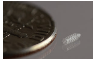
Machined prototype made in a bioabsorbable resin
