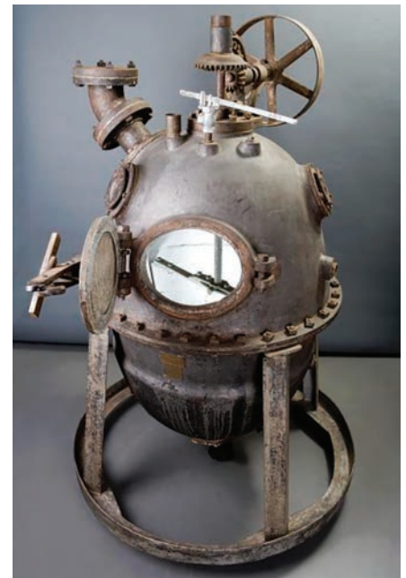
FIG. 2. The Bakelizer, the pressure vessel Leo Baekeland used to produce the world's first synthetic plastic. Photo courtesy of the U.S. National Museum of American History (Smithsonian Institution).
