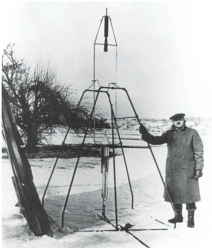
FIG. 5. Goddard standing next to his rocket. On March 16, 1926, he successfully launched the world’s first liquid-propellant rocket. Photo courtesy of the U.S. Smithsonian National Air and Space Museum.
