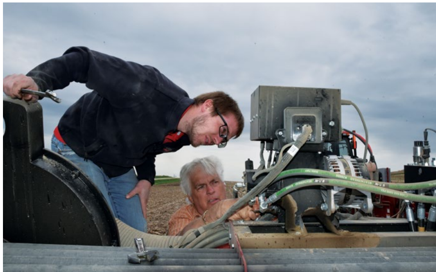
Wrench in hand, Pete Kopriva attempts to pinpoint the source of an oil leak on the alternator of a customer's Case IH 36-row Early Riser 1265 planter.
