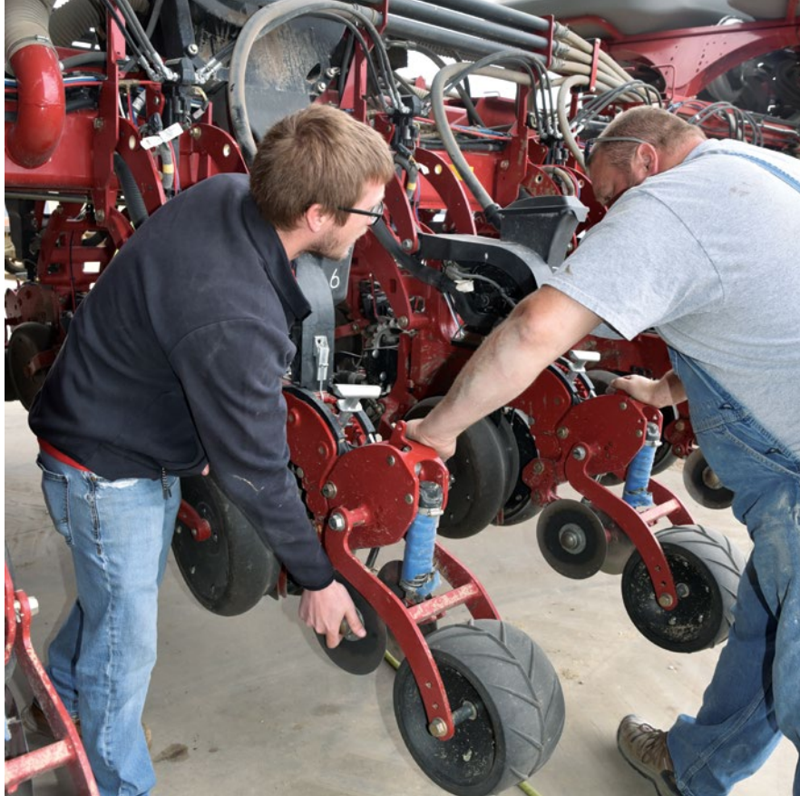
Pete Kopriva and Ryan, a customer who farms nearly 5,000 acres in the West Liberty, Iowa, area, take a closer look at row unit 6, which had a downforce issue caused by a broken wire.
