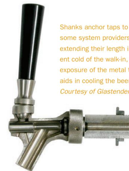
Shanks anchor taps to walls and some system providers recommend extending their length into the ambient cold of the walk-in, reporting the exposure of the metal to cold air aids in cooling the beer to the tap. *Courtesy of Glastender.*
