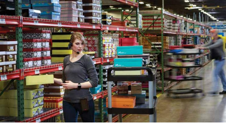
Voice-picking technology, like that of Lucas Systems, provides a heads-up picking experience with audio prompts and feedback via a headset and connected mobile device.
