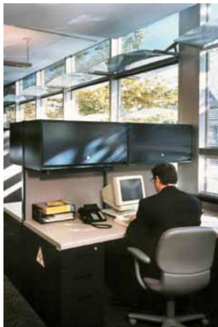
EXAMPLE OF DAYLIGHT GLAZING THAT IS SEPARATED FROM VISION GLAZING WITH A LIGHT SHELF. IMAGE COURTESY OF BP+W
