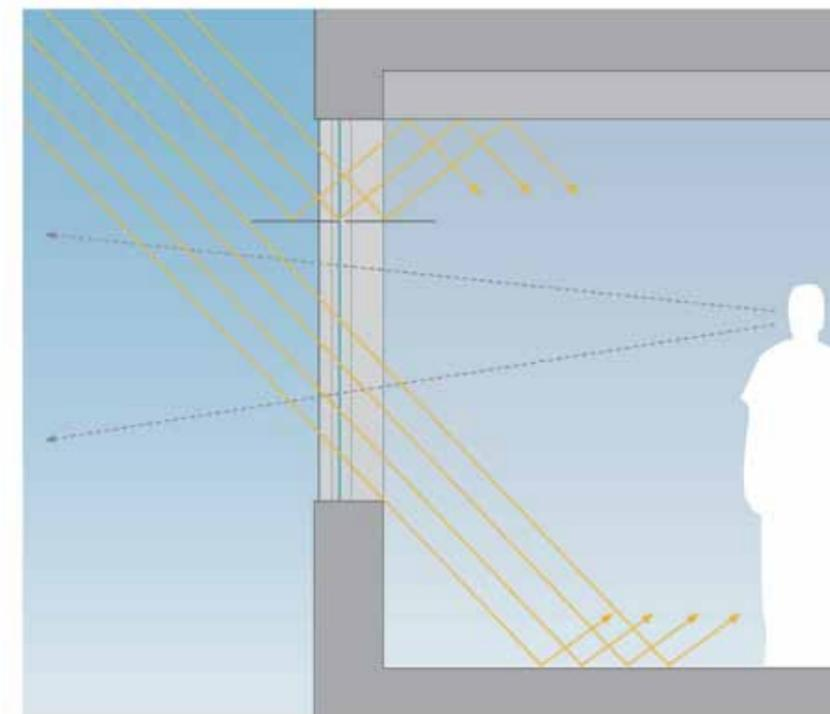
SECTION DETAIL SHOWING INTERNAL AND EXTERNAL FIXED SHADES ASSISTING IN PASSIVE GLARE CONTROL. IMAGE COURTESY OF BP+W
