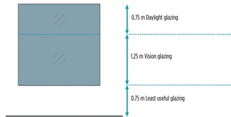
GLAZING BELOW 0.75M ADDS ALMOST NO USABLE DAYLIGHT TO A SPACE WHILE GLAZING ABOVE 2M IS THE MOST EFFECTIVE. IMAGE COURTESY OF BP+W.
