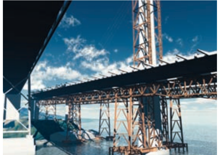
Schematic of the deck and tower erection (Klohn Crippen Berger)
