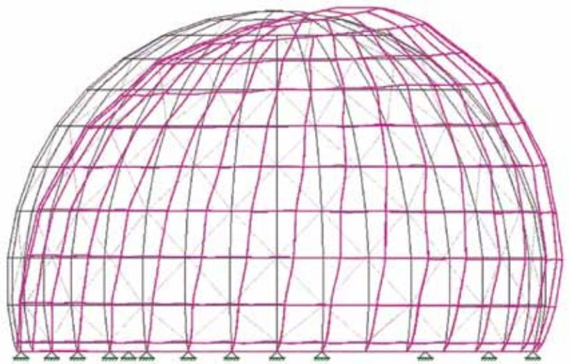
**Rain Forest Bolla's Deformed Shape under a Seismic Load**
