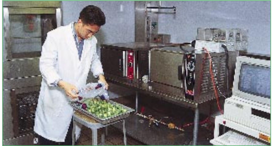
Energy usage is the biggest single component of lifecycle cost projections. Third-party data, gathered during a standardized ASTM test, help. Here, three-pan steamers are put through their paces.
